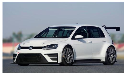
metres wider than a production Golf, and a striking rear wing giving it that ‘ready-to-race’ appearance. The 2.0-litre turbo engine with direct fuel injection comes from the top-sporting model, the Golf R.
